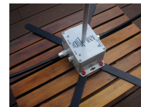
DETAIL SHOWING THE FEET DEPLOYMENT AND COAX CONNECTORS FOR THE TWO BAND SEGMENTS.
