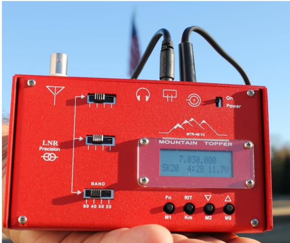
The LNR Precision MTR transceivers are designed to be efficient portable CW rigs. Whether climbing a mountain and operating SOTA or just out for an afternoon in the park, the MTR's small size, light weight and meager battery requirements makes it a great choice for these activities.
